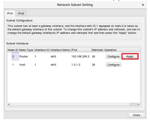
11. Configure other Node Interface IP which could not be duplicated to physical network IP.
