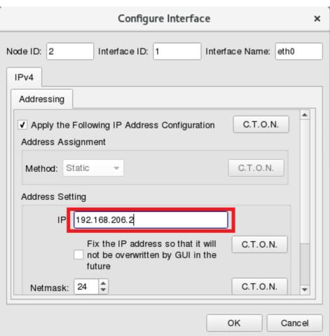
10. To make the same subnet between simulation Node and a physical network interface card.
