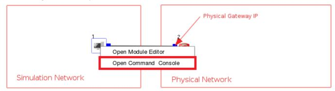
15. Use command "ping" to test the network connection status. PS. IP 8.8.8 is Google DNS server.
