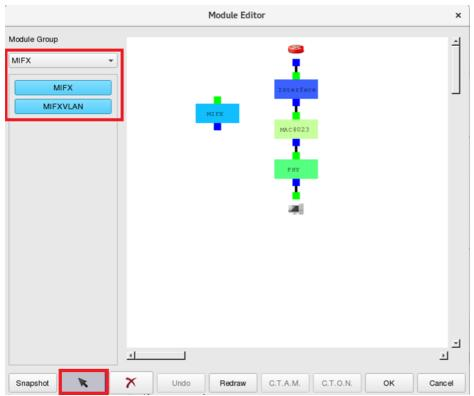
Remove the connection between module" Interface" and "MAC8023".
