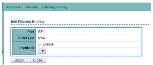
Figure 11-13 Edit Multicast Filtering Binding page
