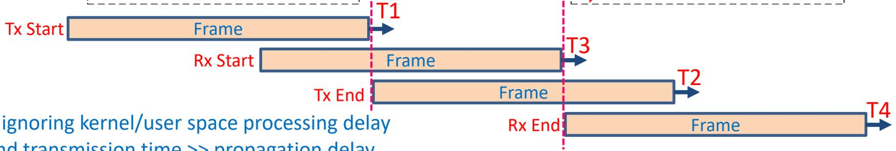
If ignoring kernel/user space processing delay and transmission time  $\gg$  propagation delay, transmission time dominates end-to-end delay.
