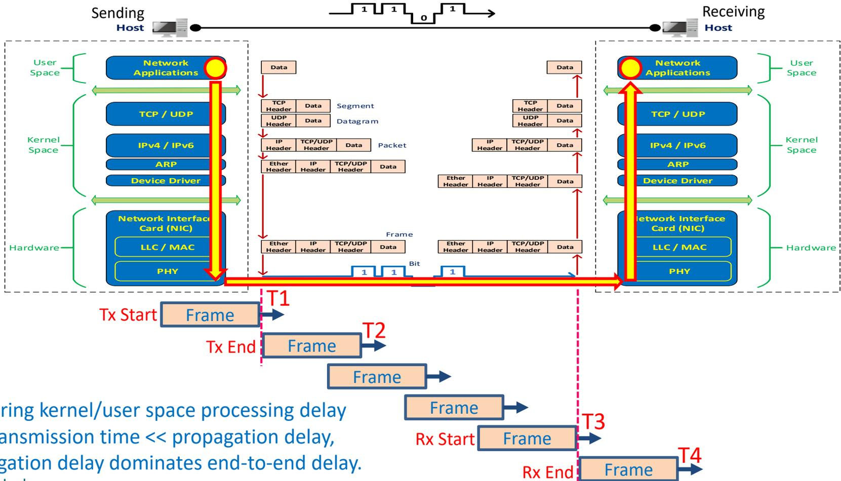
If ignoring kernel/user space processing delay and transmission time  $\ll$  propagation delay, propagation delay dominates end-to-end delay.
