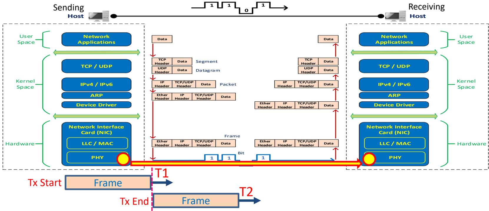
Sending Host's Interface Data Rate =  $X \text{ Mbps} = (X * 10^6) \text{ bps}$
