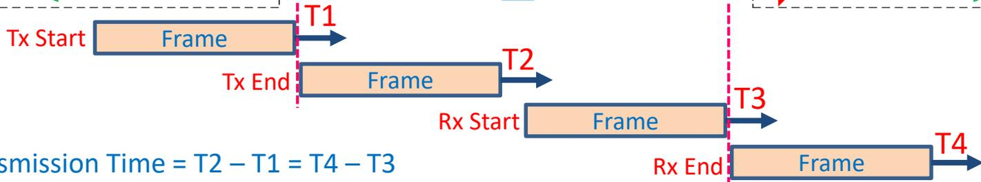
$$\text{Transmission Time} = T_2 - T_1 = T_4 - T_3$$
